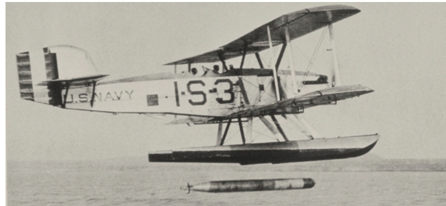
The SC-2 dropping its torpedo from a height of 12 feet. Martin built 40 of these torpedo-bomber-scout planes, underbidding Curtiss for the production contract, 1926.
