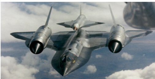
In the 1960s, Skunk Works developed the ramjet-powered, high-altitude D-21 reconnaissance drone sitting atop an SR-71.
