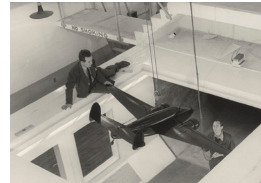
Electra wind-tunnel testing of additional fins near the end of the tailplane, 1941.
