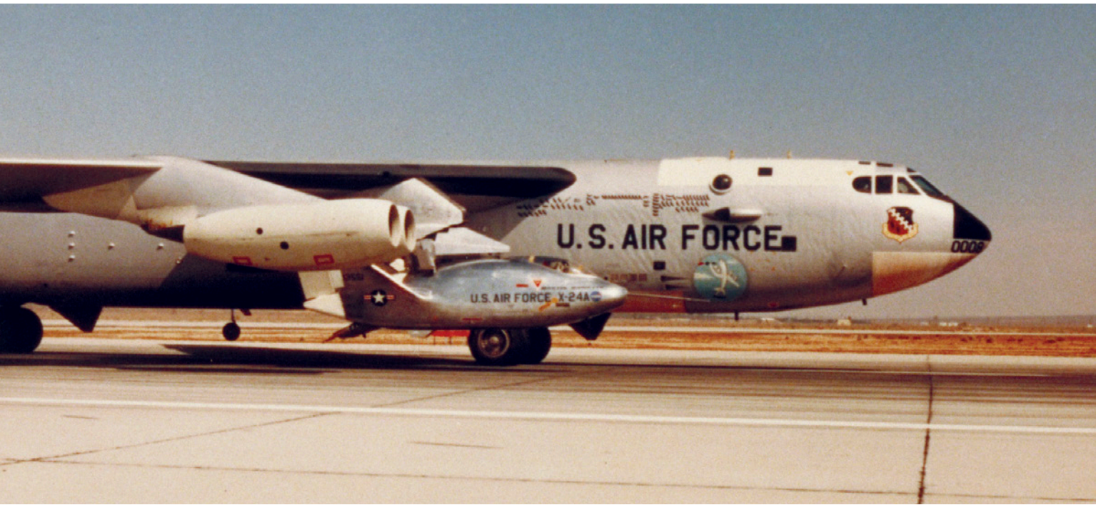
Martin Marietta's rocket-powered X-24A lifting body research vehicle is fixed under the wing of a B-52 mother ship, preparing for a test flight, c. 1970.
