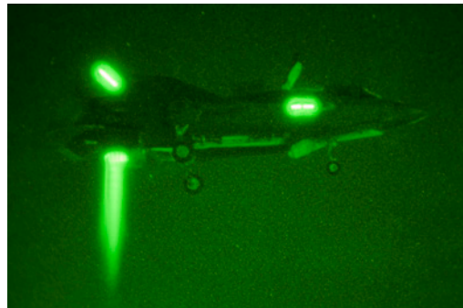
Using energy generated by the aircraft’s single engine, a swiveling jet pipe capable of rotating 95 degrees in 2.5 seconds can redirect the engine thrust downward, while the lift fan, behind the cockpit, produces 40,000 pounds of vertical thrust. Here, an F-35B STOVL aircraft hovers during a night test flight, Dec. 13, 2012.
