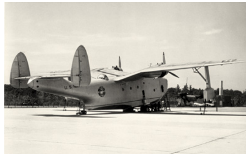
The XPBM-1 (Model 162) Mariner prototype. The horizontal tail was changed to the upswept pinwheel tail after flight testing. More than 1,300 of the patrol bombers were built in several variants for the U.S. Navy, 1939.
