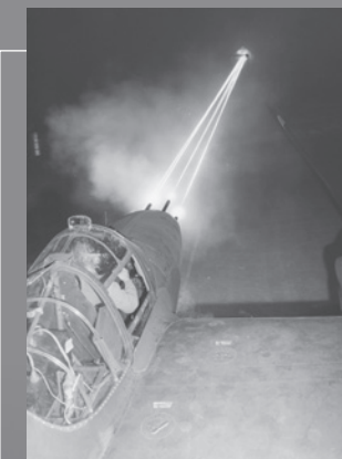
P-38 machine gun firing test, with .50-caliber machine guns firing a tracer with every fifth shell, 1941.
