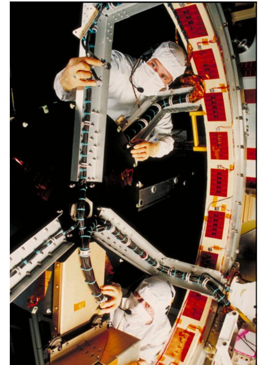
It cost Lockheed $30 million to provide a clean room that would ensure that Hubble's optics and instruments were free of dust, filtering out particles as small as 1/50th the width of a human hair.
