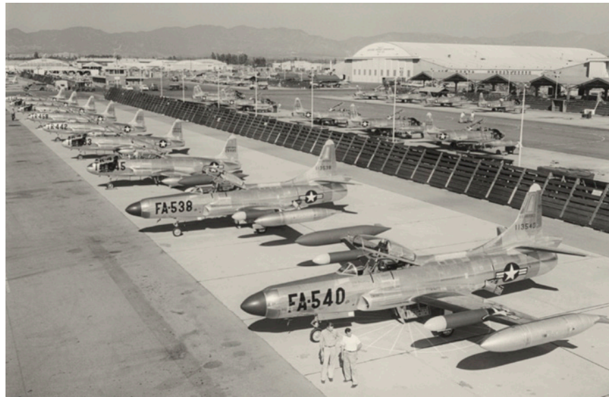
The F-94C Starfire variant was reconfigured to accommodate many updated features, including nose-mounted rockets, an automatic pilot system, closed-breech launchers and drag chute for reduced airframe stress during landing, 1953.
