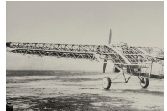
Built in the early 1920s, an uncovered Martin MO-1 showcases an all-metal framework. The wing shows certain structural similarities to the Vega's cantilevered approach, but the aluminum alloy materials were a striking departure from the Vega's all-wood construction.
