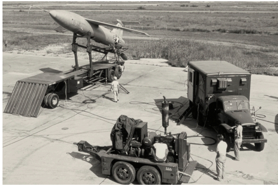
The Martin Matador offered significant breakthroughs in propulsion, guidance and launch procedure. It was propelled by a turbo jet for cruising in flight and a solid rocket booster that ejected from the aircraft's body after launch.
