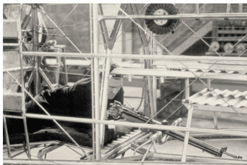
The T4M-1 radio operator had a rear-firing ventral machine gun, shown here in the fuselage framework, 1928.
