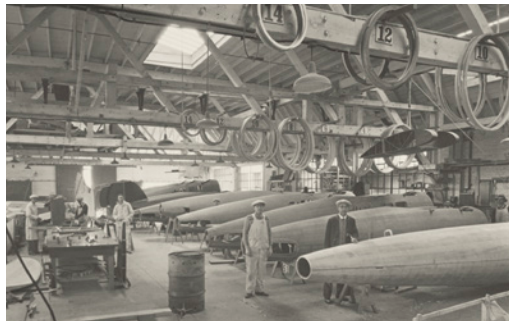
Assembly line with Vega monocoque fuselages in the early production days in Burbank, Calif., 1930.
