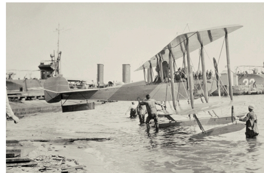
The Model S Hydroplane was a single-float sea plane version of the TT. With two destroyers in the background, Navy personnel help guide the S into the water. Note the expanded gap between the fuselage and the lower wing.
