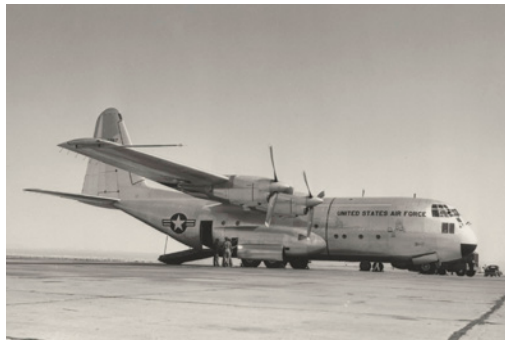
The prototype YC-130 had a cargo deck that was capable of carrying an astonishing 300 pounds per square foot, lifted into the air after a ground roll of a mere 855 feet.
