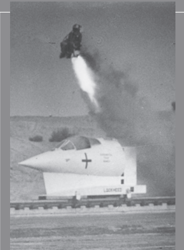
A pilot ejects via a rocket-propelled cockpit seat from an F-104 rocket test sled at Edwards Air Force Base, 1950s. Ejection seats greatly reduced the number of pilot casualties.
