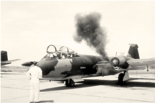
A B-57B Canberra, upgraded and camouflaged for operations in Vietnam, emits smoke during a normal cartridge-starting procedure. Only 36 B-57s, many of them unpainted, were used in Vietnam, 1968.
