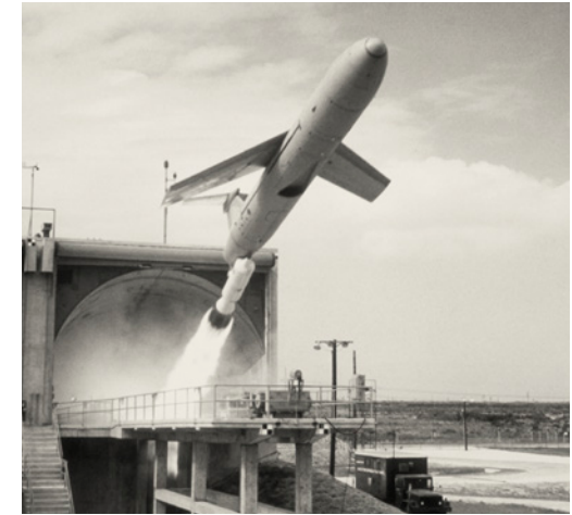
A TM-76A Mace missile, successor to the TM-61 Matador, launching from a dual-missile shelter, 1960.
