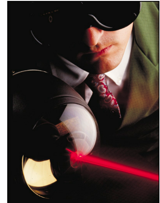
The Hellfire missile system seeker homes in on a laser-illuminated target in the laboratory. The Hellfire is an air-launched antiarmor missile, the primary armament for the Army AH-64 Apache.
