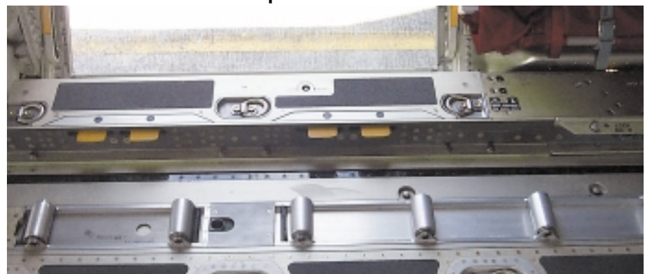
Above: A close view of an electronic lock in the locked position. Below: There are eight vertical restraints located in the aft cargo area and sixteen on the ramp.
