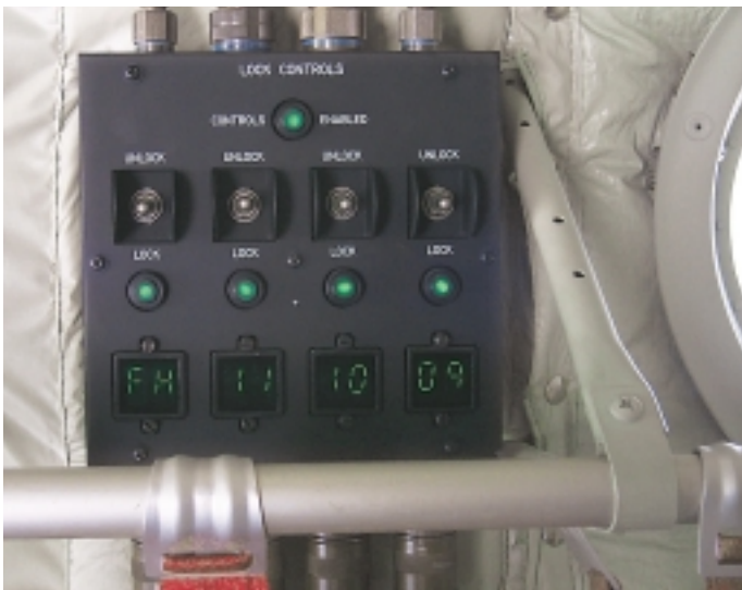
The Pallet Lock Control Units are strategically located in the cargo compartment.
