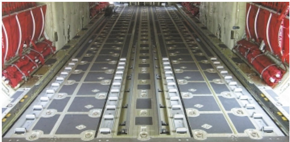
In this photo, the aft portion of the cargo compartment is configured with rollers and center vertical restraints.
