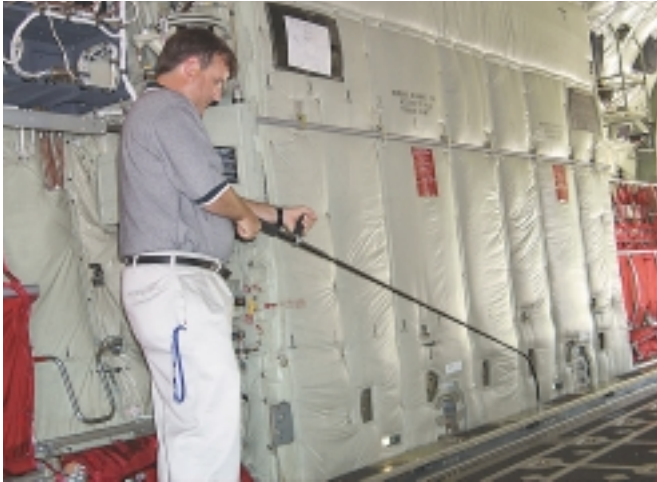
In addition to the standard manual tool, a long reach tool is provided for manual actuation of the locks when the cargo compartment is full.
