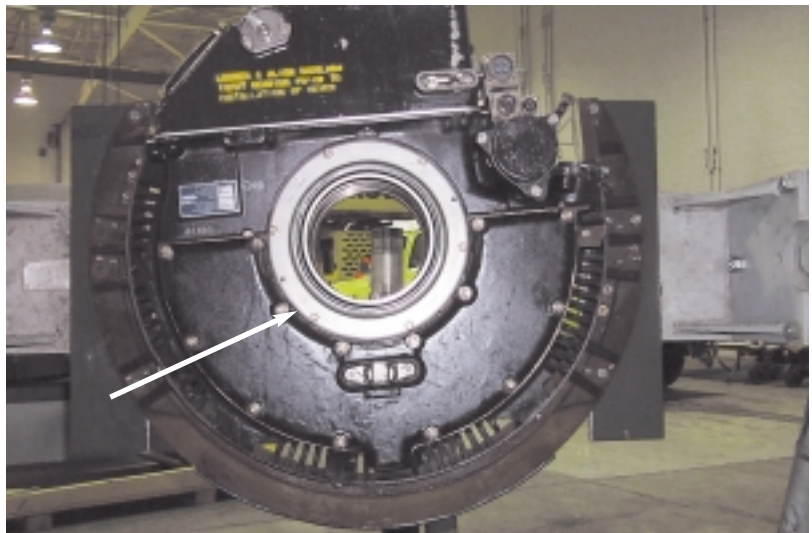
Pump housing rear lip seal.
