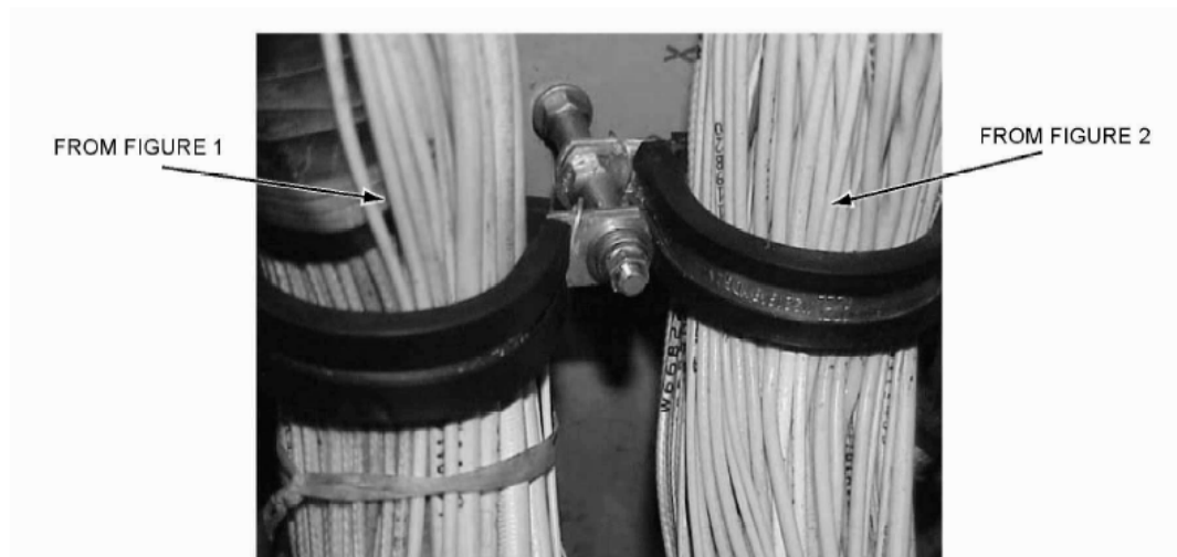
Modified Wiring Bundle Assembly Figure 3
