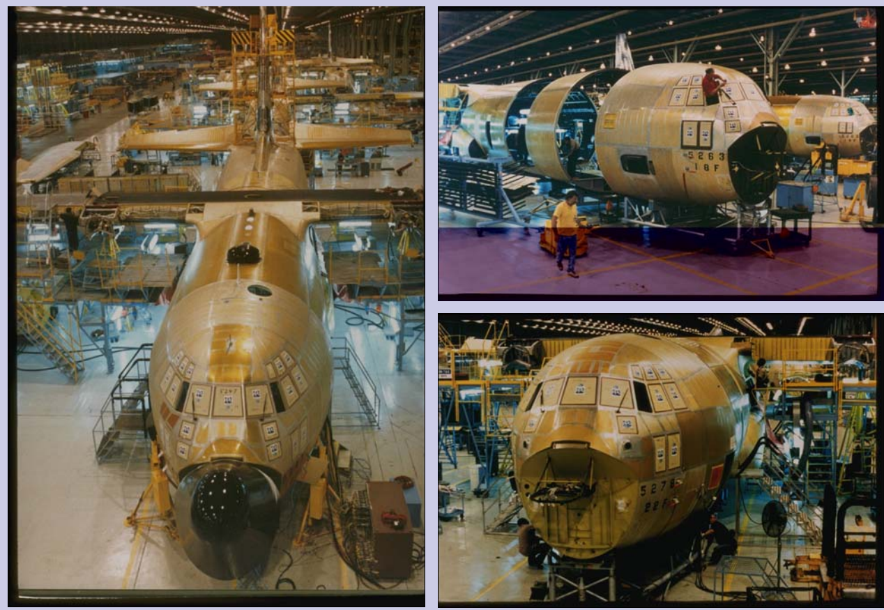
The Lockheed – Georgia manufacturing line for the C-130 aircraft. Images—Lockheed Martin Archives
