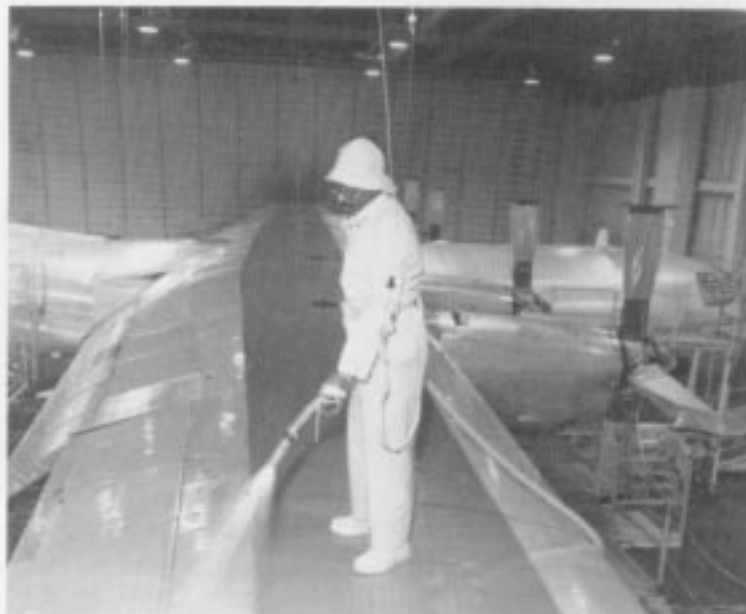
Washrack workers need the protection of safety harnesses when working on the upper surfaces of the aircraft.
