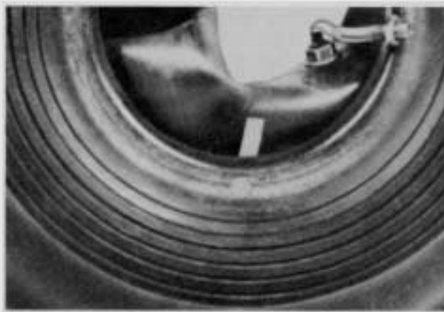
Tube balance mark (heavy point) aligned with tire balance mark (light point). Photo courtesy of B F Goodrich Co.
