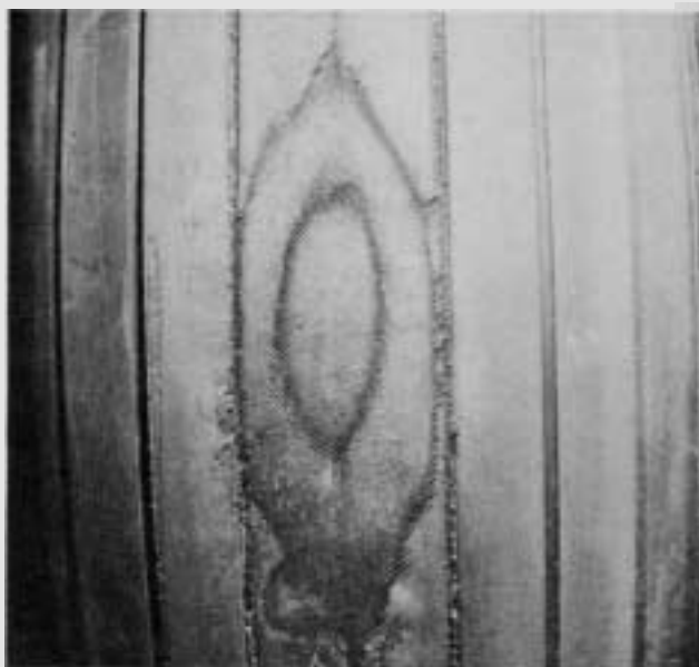
Worn through tread reinforcement strips only. O K for retread. Photo courtesy of B F Goodrich co.
