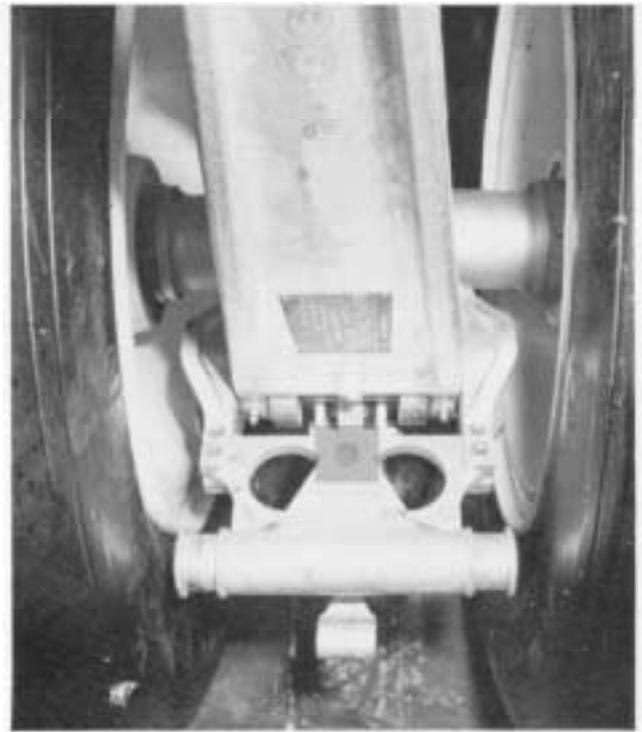
Figure 1 A SHEAR BOLT SECURES TOW FITTING TO CROSS BAR ON NOSE LANDING GEAR.
