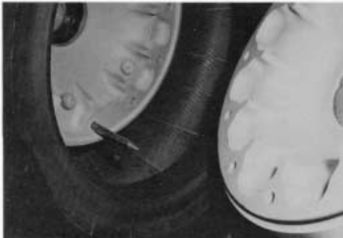
Guide pin used for alignment of wheel halves.
