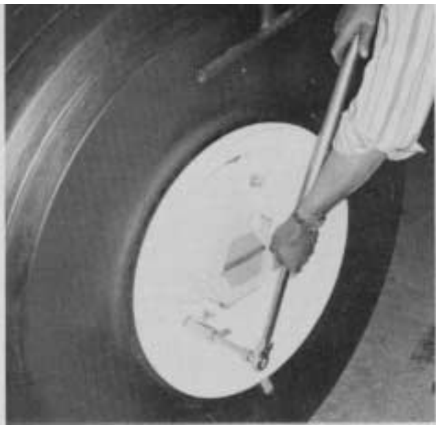
Tightening wheel bolts with torque wrench
