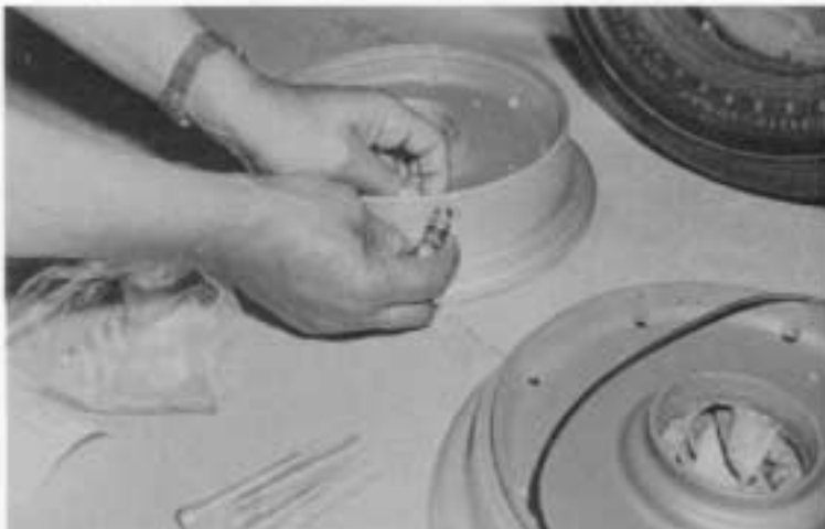
inserting valve stem into wheel.
