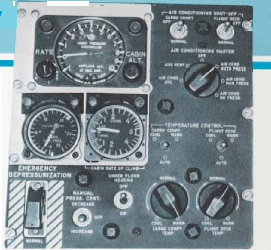
AIR CONDITIONING CONTROL PANEL
