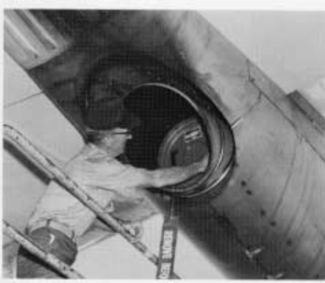
Above: Engine tailpipe plug being installed to prevent entrance of contaminants. Below: Waterproof adhesive tape and sheet material are used to prevent damage by cleaning solutions during washing. Openings are closed, plastic areas are covered and the landing gear is shielded with these materials.
