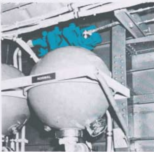
PHOTOGRAPH OF ENCLOSED AREA ABOVE LEFT MAIN WHEEL WELL. HIGHLIGHT SHOWS LOCATION OF THE GROUND TEST INTERCONNECT VALVE ON PRODUCTION HERCULES SINCE A CHANGE IN 1965. VALVE IS ACTUATED MANUALLY BY CABLES FROM A HANDLE LOCATED IN THE LEFT WHEEL WELL FAIRING. EARLY HERCULES HAD TWO INTERCONNECT VALVES DIRECTLY BEHIND THE HANDLE.
