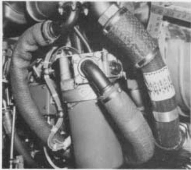
FIGURE 3. (above) A differential pressure (clogged filter) indicator is integral to the filter assembly. FIGURE 4. (right) It is difficult to install the element upside down – remember the tang end goes up. Sometimes stamped with the word “top”.
