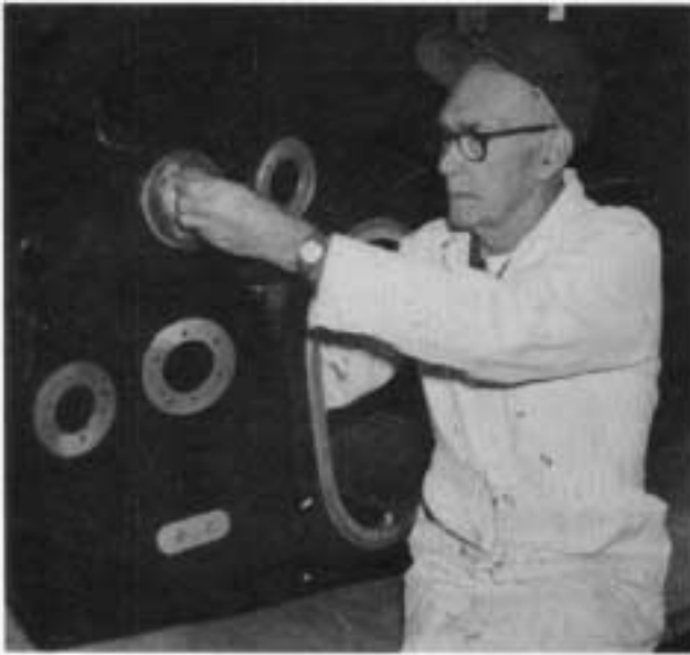
Rubber gaskets on plates cover openings, including bolt holes, to make bladder cells air tight. Cords suspended above work platform position bladder cell for inflation. A manhole cover provides connections for a manometer and air pressure. The cell below is inflated at 1/2 psi.
