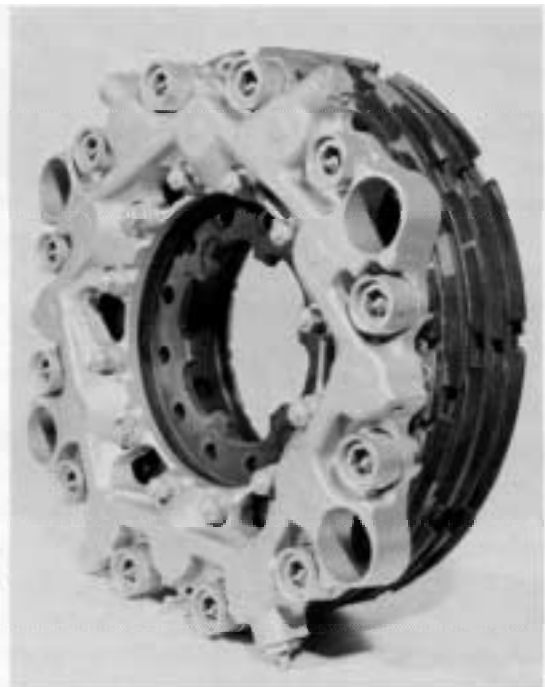
Single Disk Brake Provided on Early Hercules Models
