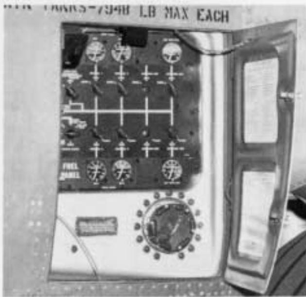
A typical fuel control panel, accessible from the ground, for fuel transfer between tanks, as well as for fueling and defueling the Hercules.
