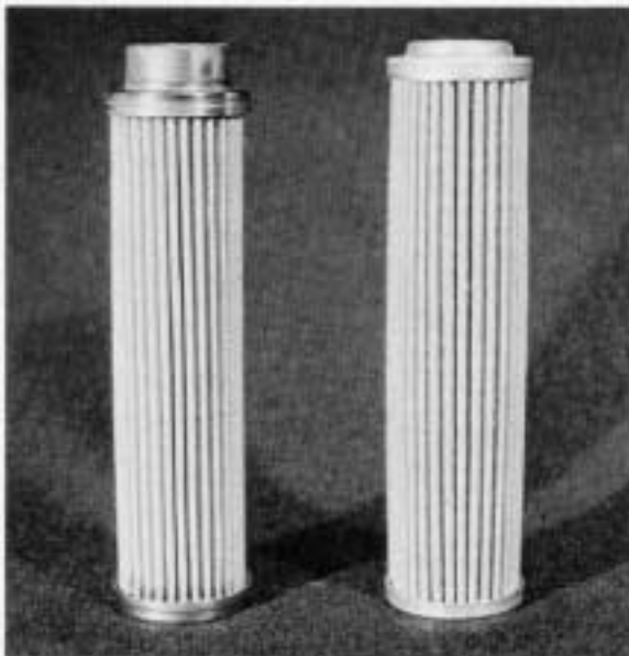
Filter element at right is typical of the ones previously used in the subject hydraulic systems. The element at left is a new one. The outer protective wire screen is a distinguishing feature. Part numbers are stamped into the bottom of each element.
