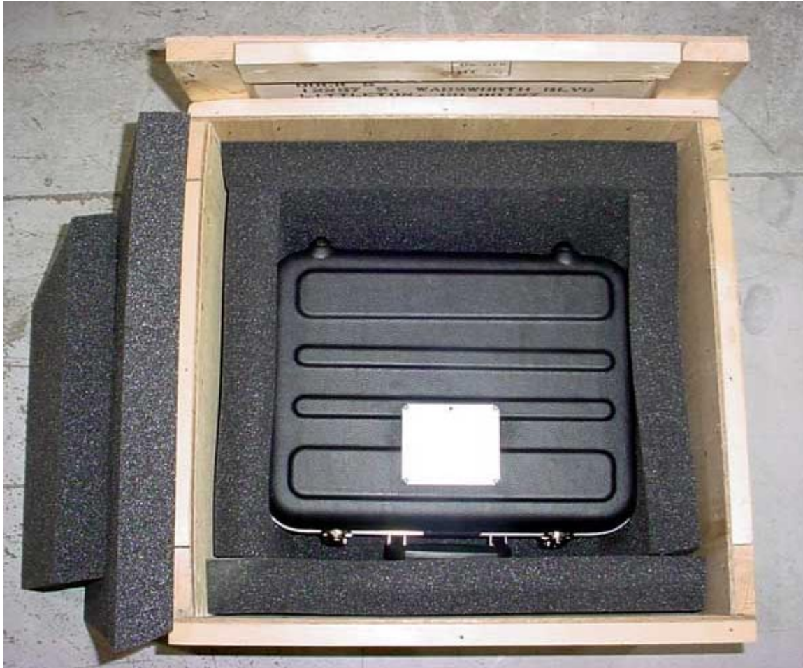
Figure 2. Delicate Product/Equipment – Wood Box Overpack
