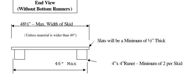
46" – Maximum Spread of Runners Measured from the Outside of One Runner to the Outside of the Next
