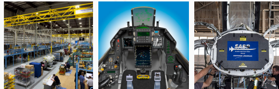
1. Left Photo: F-16 Production Line in Greenville, South Carolina 2. Center Photo: New Advanced Block 70/72 Cockpit 3. Right Photo: APG-83 Active Electronically Scanned Array (AESA) Radar
